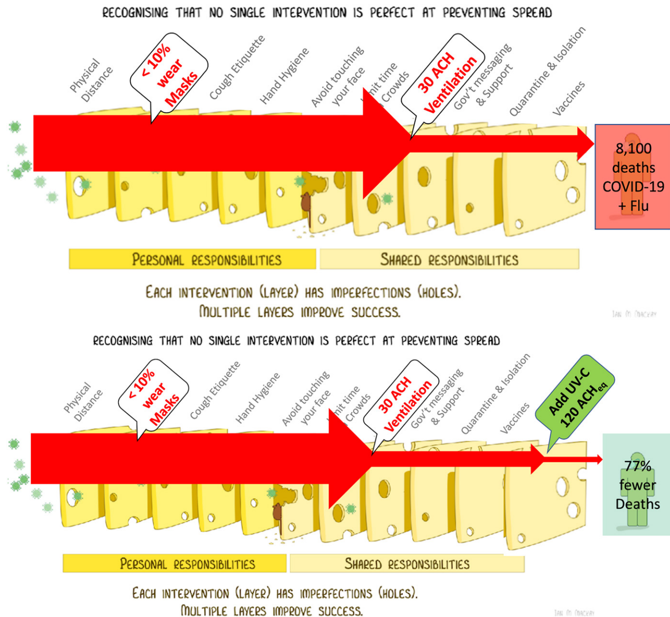
Fig. 4. ICAO Aviation Multi-Layered Disease Defense Strategy. Top: without UV-C air disinfection layer added. Bottom: with UV-C air disinfection layer added.
